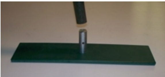
Mast pole places over plate with plug.
