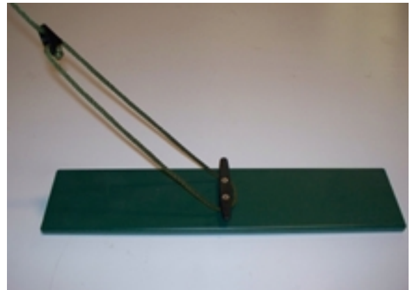
Guy lines go over plates with cleats.
